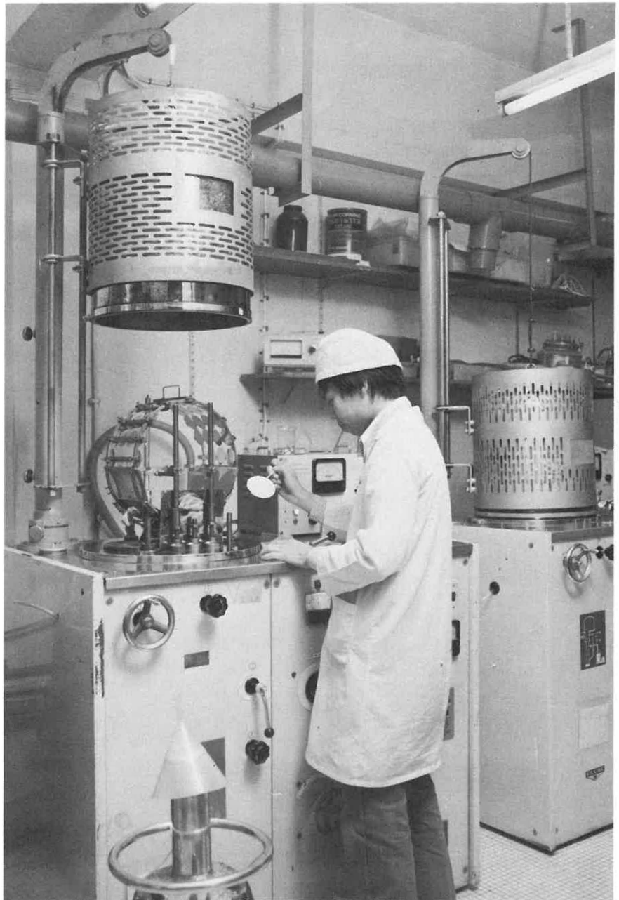
The TIC actively encourages new industrial ventures — whether of domestic or overseas origin. Picture shows high vacuum evaporation machines for production of silicon wafer chips.
